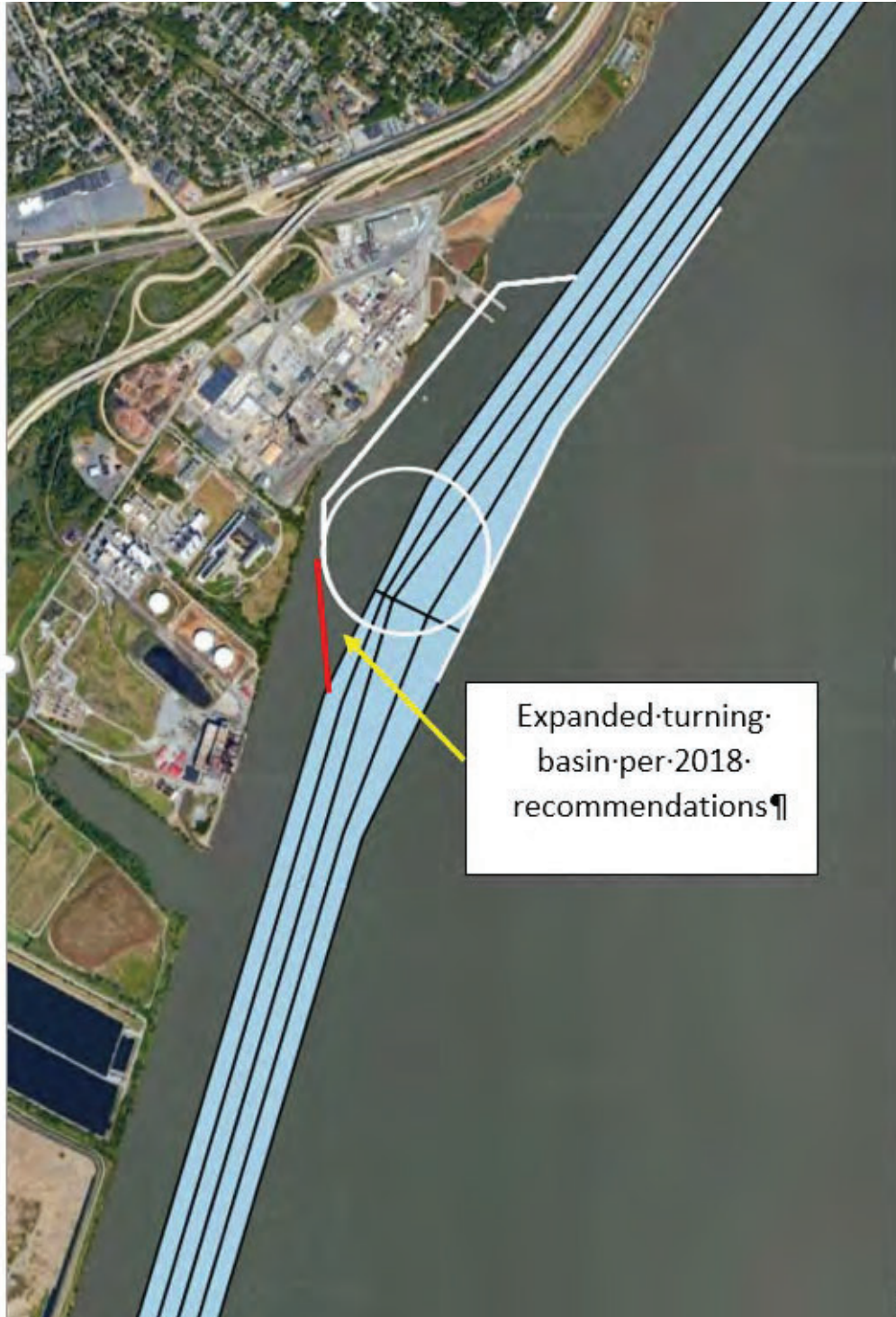
Figure 3-2: Existing Main Navigation Channel Overlaid with Proposed Berth Pocket, and Expansion of Turning Basin depth to 45 ft. from 2018 Design Consideration Comments.
